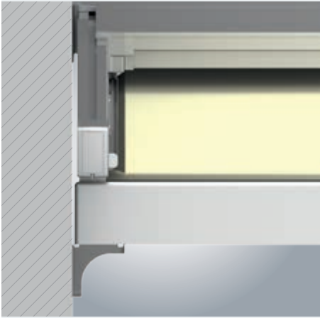
Installation of the guttering laterally on a wall using the guttering angle bracket
