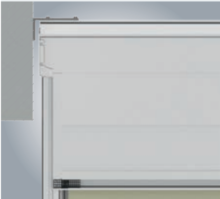
Installation laterally on a wall or in a niche using the 200 x 100 x 10 x 140 mm angle bracket
